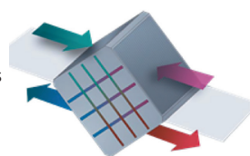
Plate cross-flow heat exchanger operating logic
